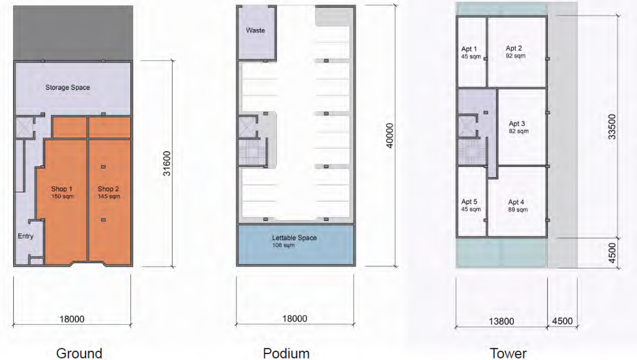
Figure 13: 18 metre frontage outcomes and car parking setback options in higher density built form
