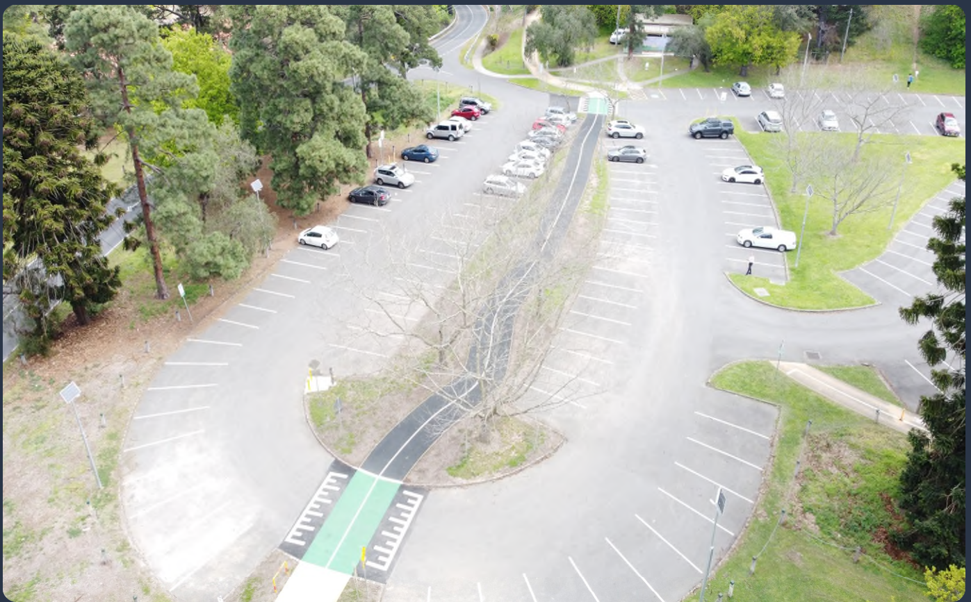
Figure 16 | Shared user path constructed with Porous Lane at Heidelberg Park
