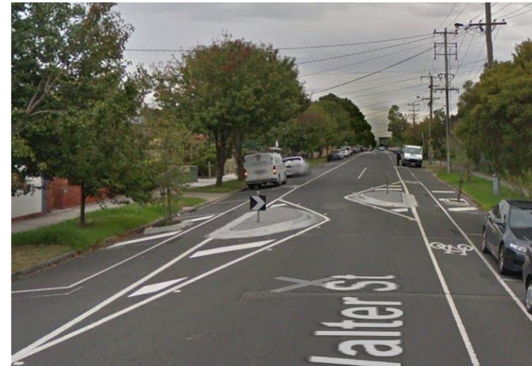
Slow point with cycle bypass, Footscray VIC
